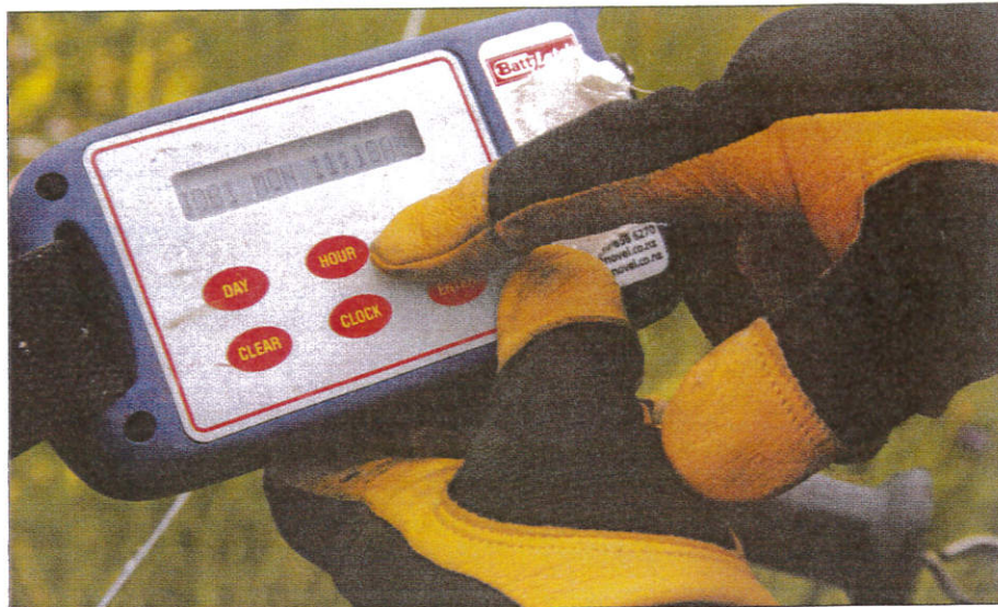
Using a Batt-Latch allows grazer Neil Dennis to set his gates to automatically release, allowing his cattle access to fresh pasture without manual labor.
